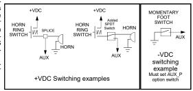
Cutout Input Connection - The Cutout Input turns off any siren tone output when activated, and remains off until a control is activated or changed. The adjacent diagram shows two connection examples. See OPTION SWITCHES section for programming details.
